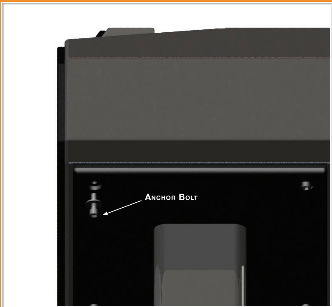
FIGURE 11 - BOLTING THE CENTER CHANNEL TO THE STAND
